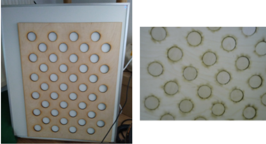
Figure 4.4: Heating the calibration pattern (left) and calibration layout after heating (right)
