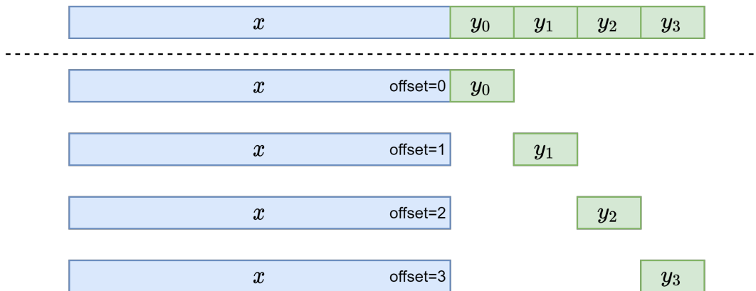
FIGURE 5.2: The process of transforming time series with many missing values into a tabular format. For each known performance value y_i , a sample with a set of features will be present in the dataset. If a meter did not get dispatched in a given month, then the target label is not known, and therefore the sample will not be present in the dataset.
