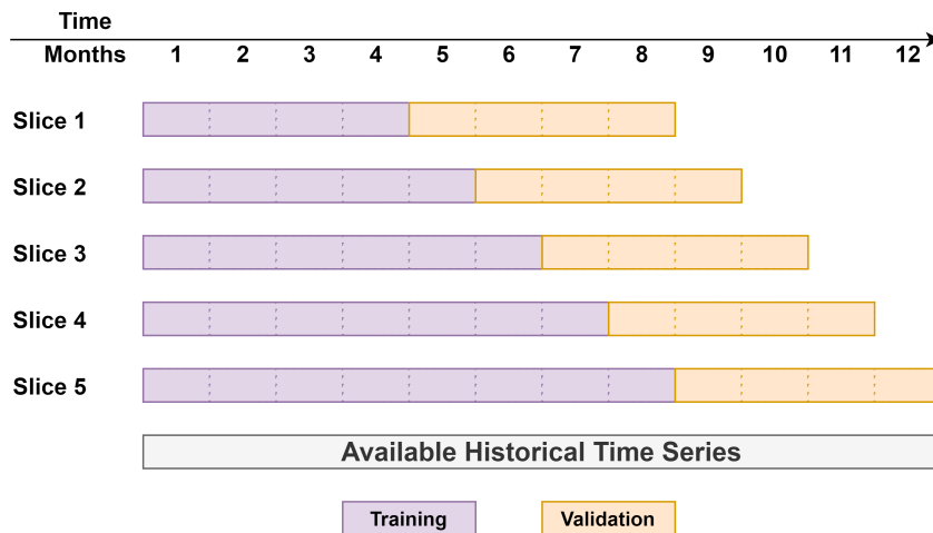
FIGURE 5.3: In the expanding window validation method, the validation sets from different slices are allowed to overlap. In the first slice, a certain time frame is used for training, and a consecutive time frame is used for validation. In each subsequent slice, we will move the training time span forward by one month, just like the validation time frame. There is no overlap between the training and validation sets within a single slice.
