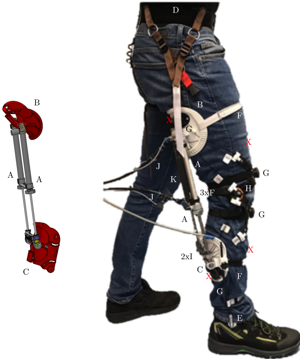
Figure 2.1: A drawing (left) and a picture (right) of the pneumatically actuated knee orthosis used in the experimental validation. The orthosis consists of two pneumatic cylinders (A) and an upper (B) and lower shell (C). To compensate for its weight, the orthosis is attached to a waist band (D) and rests on two pins attached to a shoe (E). Five velcro straps (F) and six Boa closure systems (G) attach the orthosis to the body. Two anchor points (H) are present to attach the cables from the closure systems. A load cell (I) is present for each cylinder to measure the force and a pressure sensor (J) is present in the air supply for each cylinder to measure the air pressure. One of the cylinders has a linear Hall sensor (K) to measure the piston position. The four marker frames (X) of the motion capture system, described in Section 2.5.4 are attached to both of the shells and the anterior side of the upper and lower leg.
