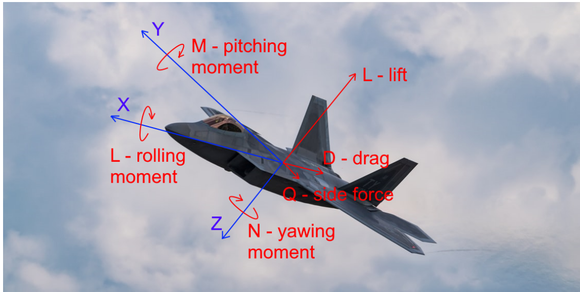
Figure 2.1: The 3 linear and moment forces that work on a UAV (North, East, Down (NED) coordinate system)
