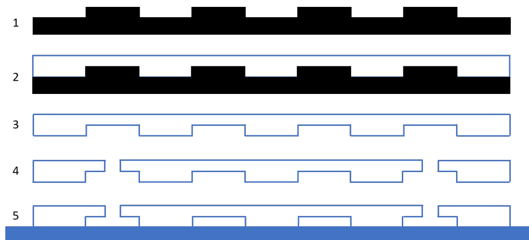
Figure 2.5: Schematic representation of the process of soft lithography to produce a PDMS microfluidic device from a 3D printed mould. 1: 3D printed mould, 2: PDMS is poured over the mould and left to cure, 3: The cured PDMS is extracted from the mould, 4: Inlets and outlets of desired size are punched into the PDMS, 5: The chip is bonded to a glass slide. Black = 3D mould, open blue = PDMS and filled blue = glass slide.
