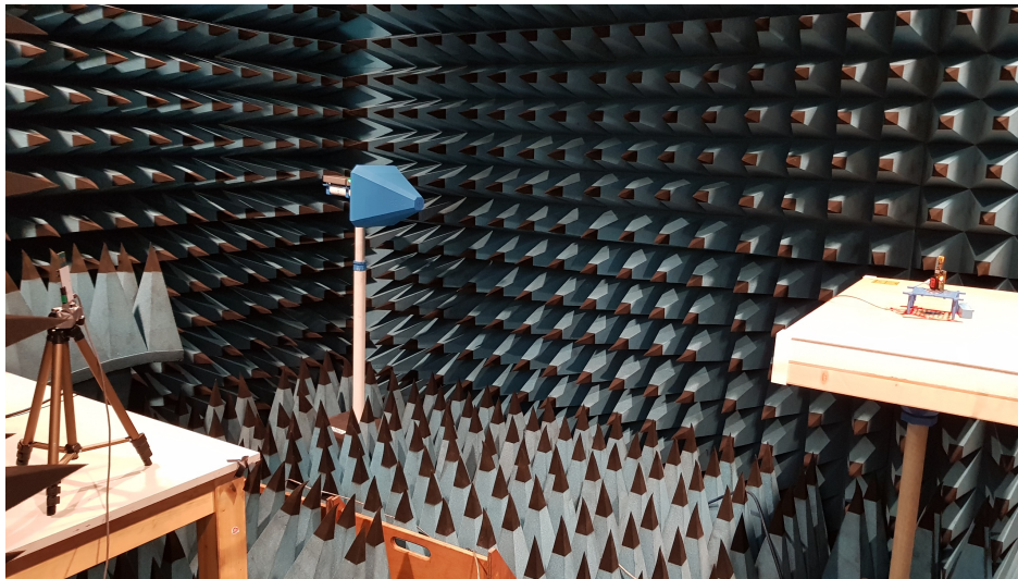
Figure 3.2: The Anechoic Chamber at the High Tech Campus in Eindhoven with the Fixed Antenna (left) and the Rotating Antenna (right).
