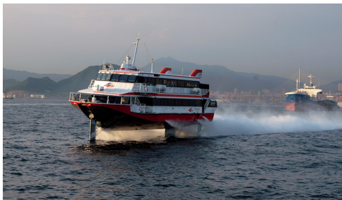
(a) Boeing 929 Jetfoil, a hydrofoil ferry from 1976 [1]
