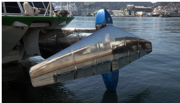
Figure 3.15: Trailing edge devices (flaps) on Jetfoil front foil [38]
