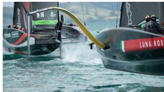
Figure 2.6: Carbon fiber composite swing-arm and hydrofoil on an AC75 racing yacht, 7.6 ton displacement [19]
