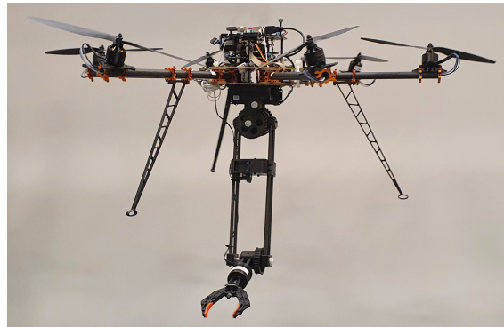
Figure 1.1: Fibrethex - a fully actuated hexarotor with manipulator.
