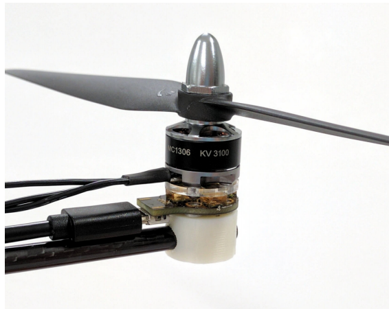
Figure 2.2: MEMs thrust sensor for micro UAVs by (10)
