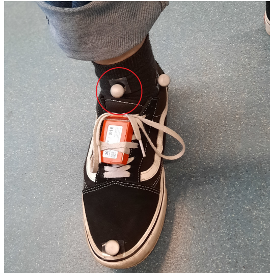
Figure 3.3: Image showing the markers added to the subject's body for tracking with Qualisys. The circled marker is used as the reference for the skeleton trackers.
