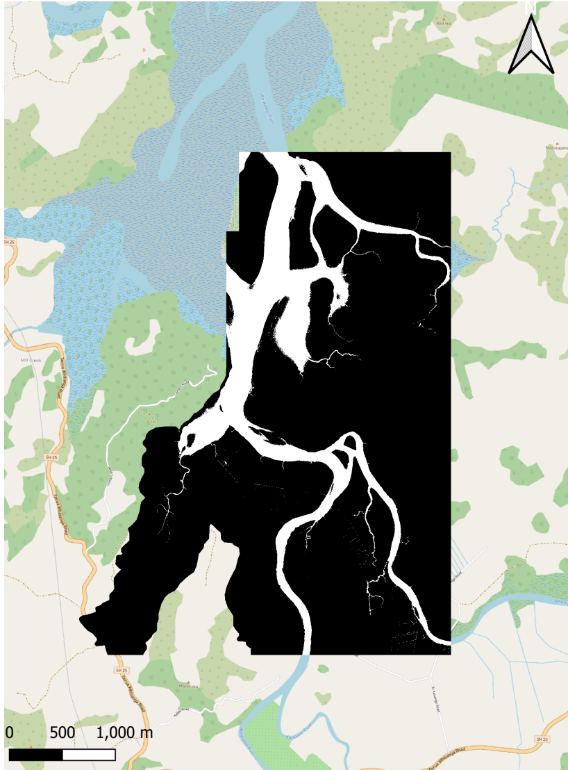
Figure 6.1: Base roughness raster with a Chézy roughness of 60 \text{ [m}^{1/2} \text{ s}^{-1}] in the creek (white) and a Chézy roughness of 2 \text{ [m}^{1/2} \text{ s}^{-1}] in the forest (black)
