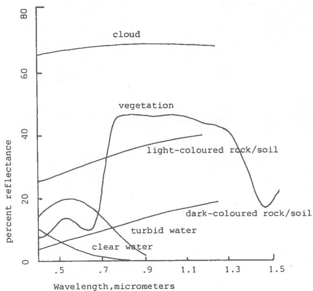
Fig. 2. Spectral characteristics of common objects
