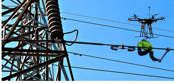
(a) A drone that has a load which interacts with a power line.
