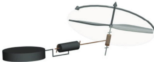
Figure 2.3: A schematic representation of a propeller that can tilt radially. [8]
