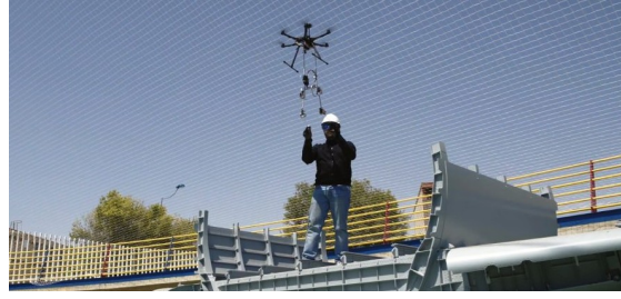
(b) A drone that holds a load and interacts with a human. (Co-working)
