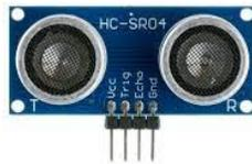
Figure 33: HC-SR04 ultrasonic sensor
