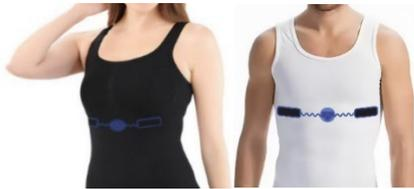
**Figure 7.;** Final Location electrodes
