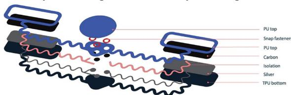
Figure 3.; Electrode layers
