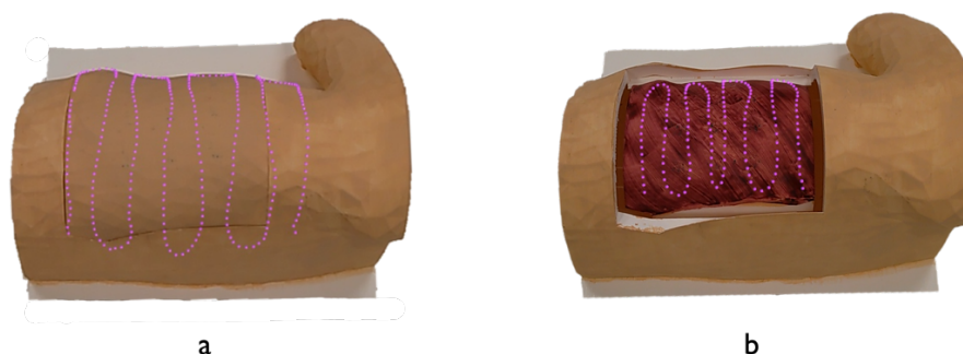
Figure 9. Example of the acquired point cloud (pink spheres) during contour registration. a) Registration pre-incision. b) Registration post-incision.
