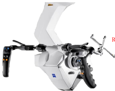
Figure 3.7: Surgical microscope integrated with the neuronavigation (R).
