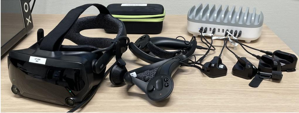
Figure 3.3: *VR headset, controllers and trackers*
