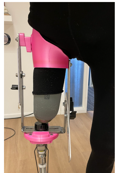
Figure 10: Set-up to evaluate the fitting of the brims using the custom-designed brim standard.
