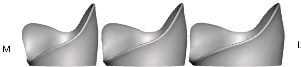
Figure 18: Anterior view of three different brim sizes from the data-supported brim set. From left to right, circumference: 40, 44, and 48 cm.
