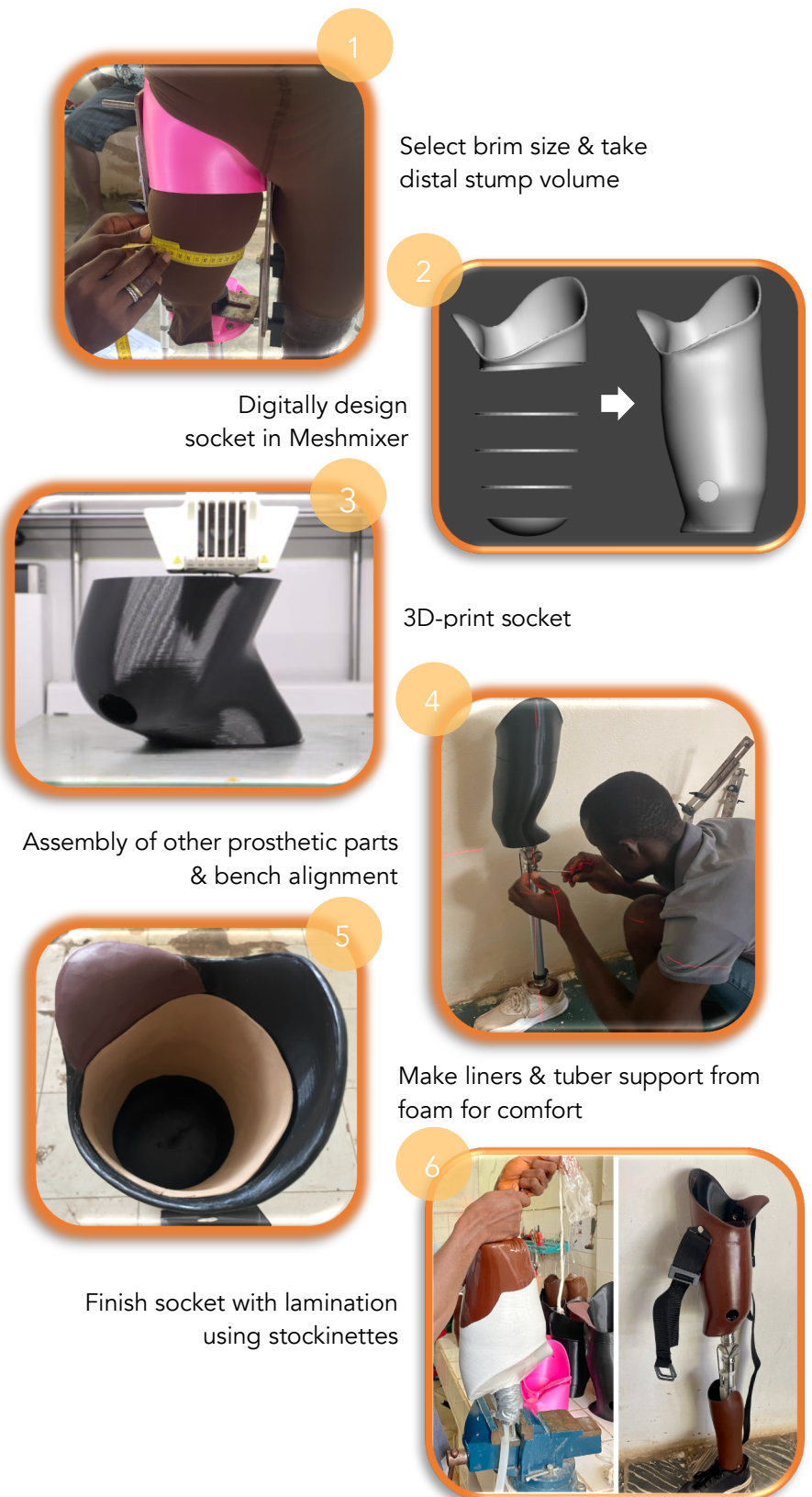
Figure 19: Flowchart showing the sequential steps taken to manufacture a hybrid TF prosthesis using a streamlined method for the socket.
