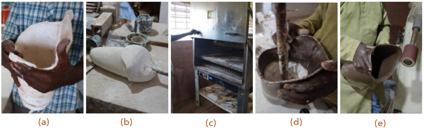
Figure 2: The traditional workflow for manufacturing TF sockets, consisting of (a) making a negative plaster model of the stump (b) modifying the positive plaster model representing the stump shape inside the socket (c) heating the thermoplastic material to cover the positive plaster model and create the socket (d) removing the plaster inside the socket, and (e) post-processing of the socket.
