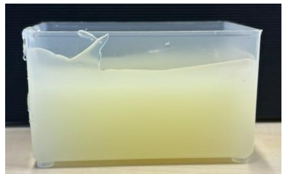
(b) the copolymer-in-oil in a cube for the acoustic measurements
