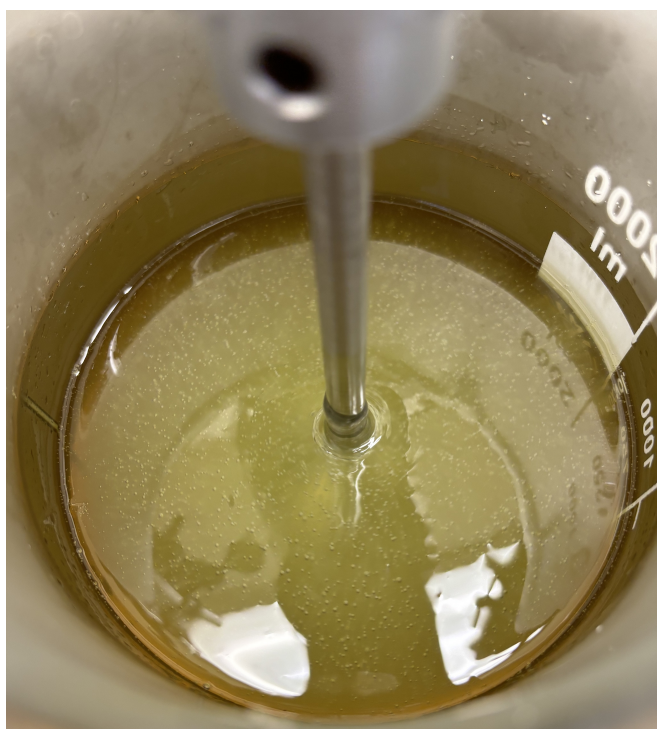
(a) The copolymer-in-oil in the oil bath, this is at about 1 hour in.
