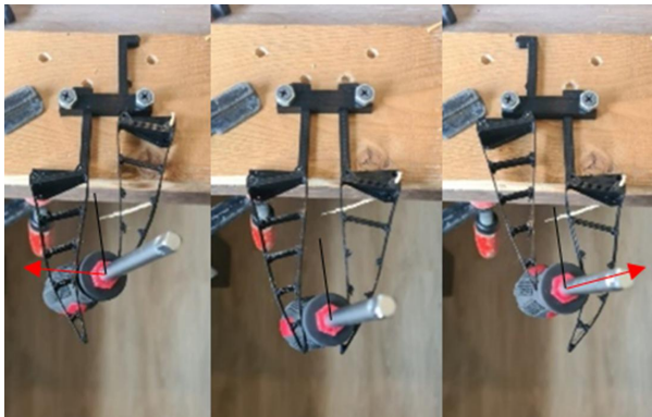
Figure 21: Initial prototype implementing adaptive grippers.
