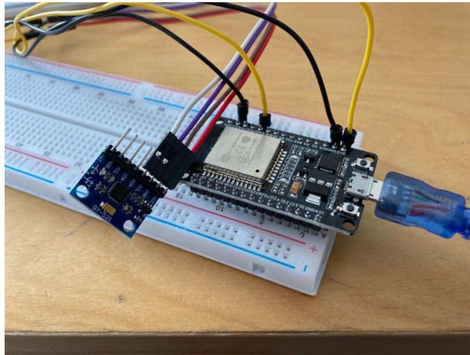
Figure 2.8: ESP-32 with an MPU-6050 gyroscope/accelerometer
