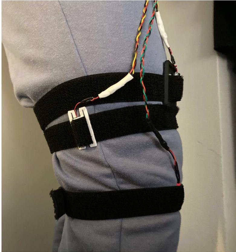
Figure 4.1: Placements of the vibration motor giving feedback on squat depth
