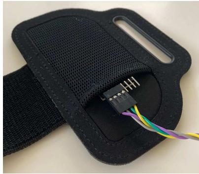
Figure 6.1: The MPU-6050 IMU in its leg strap
