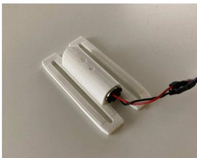
Figure 6.5: A vibration motor in its 3D-printed casing
