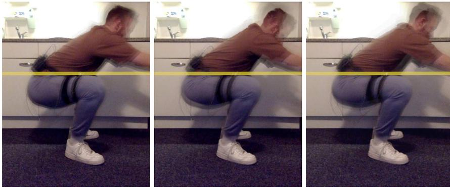
Figure 5.2: images from 3 series of 10 squats overlaid on one another to measure the squat depth sensor's accuracy
