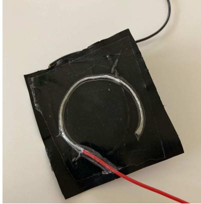
Figure 6.3: The pressure sensor made with Velostat
