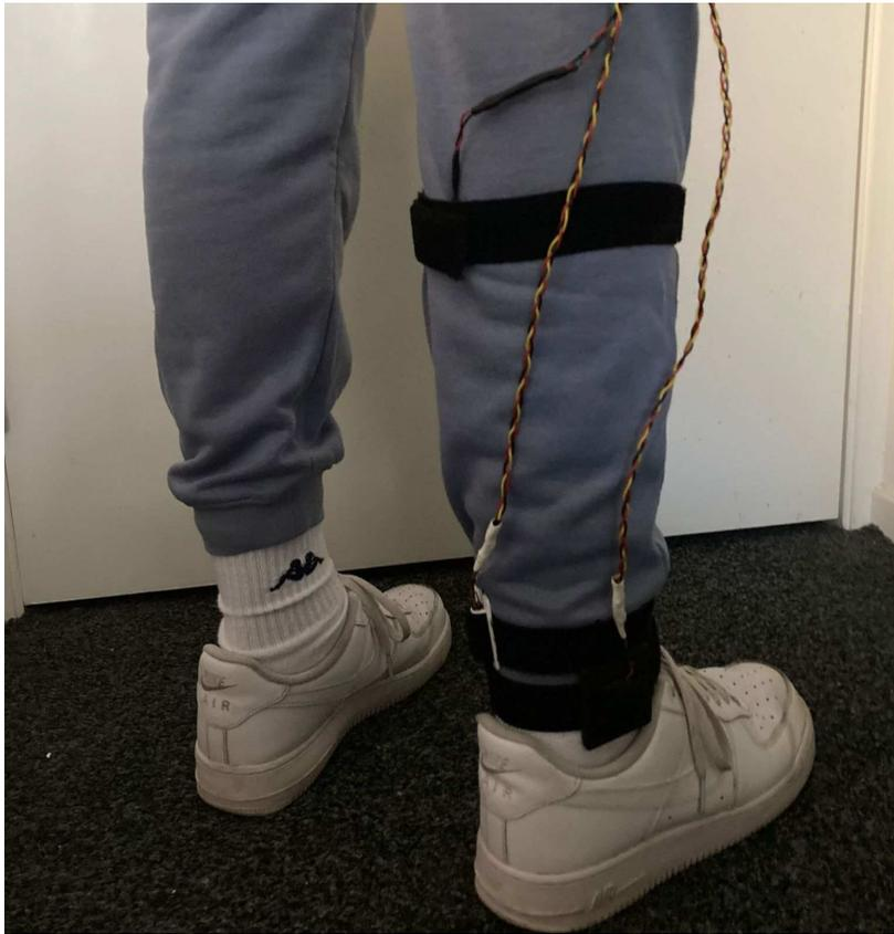
Figure 4.2: Placements of the vibration motor giving feedback on heel position
