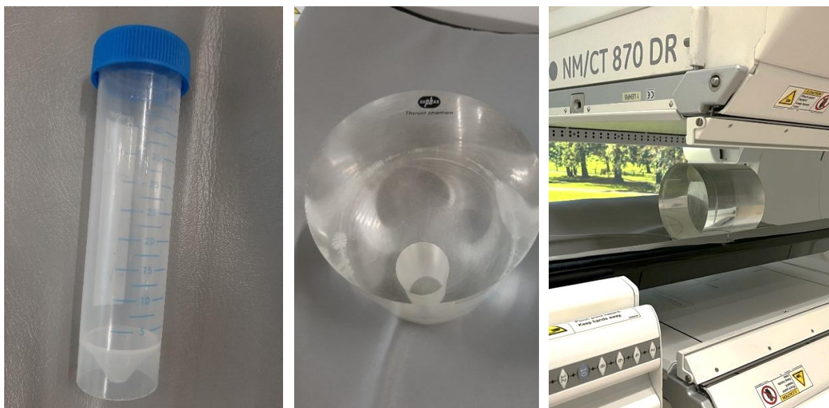
Figure 2: The 50 mL cup containing I-123 (left), the perspex thyroid phantom (middle), and the experimental set up in the gamma camera (right).
