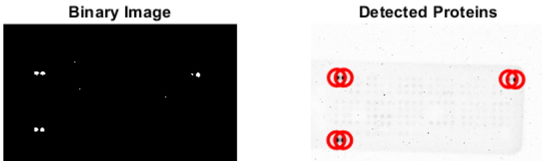
FIGURE J.3: Image processing result for detecting the reference spots within the to-be-analyzed protein array membrane (Left). Found possible reference spots marked with a red circle (Right)
