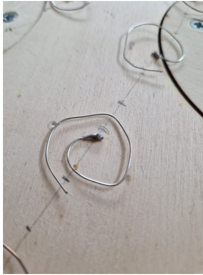
Figure 10.7: Copper wire connected to the touch pads of the Adafruit CAP1188 Breakout sensor, twisted into a circular pattern.
