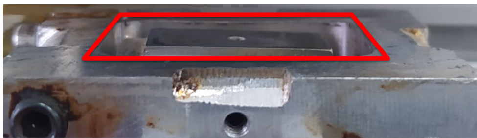
Figure 7.1: Misaligned heat block (right edge downwards) at the bottom welding head.
